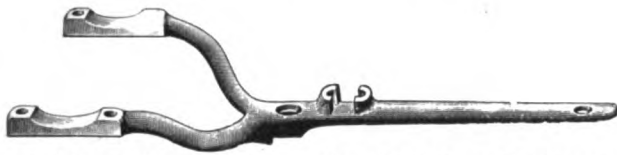
Detachable Fork Perch Connection Used in 1908 Gear Set.
